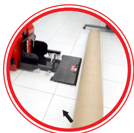
Load rolls from the ground
